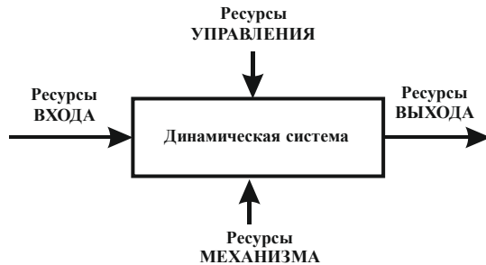
Figure 1. Diagram of the SADT model of a dynamic system
